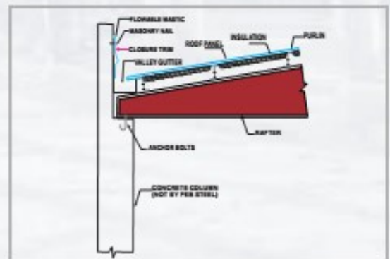
Roof system with insulation
